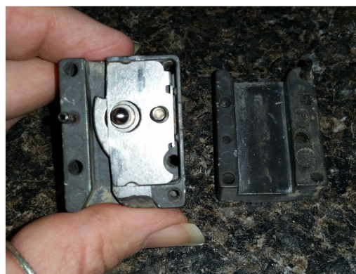
4) Clean All Parts Inside Top Block with Rubbing Alcohol
