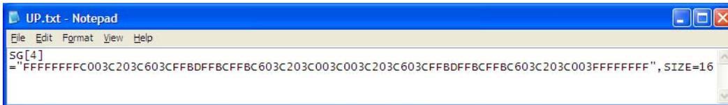
If the bitmap was manually converted to hexadecimal, the hexadecimal code should be typed in after the first quotation mark. A closing quotation mark should follow the last hexadecimal character, then the size of the graphic (16 or 32) as shown in the example above.
