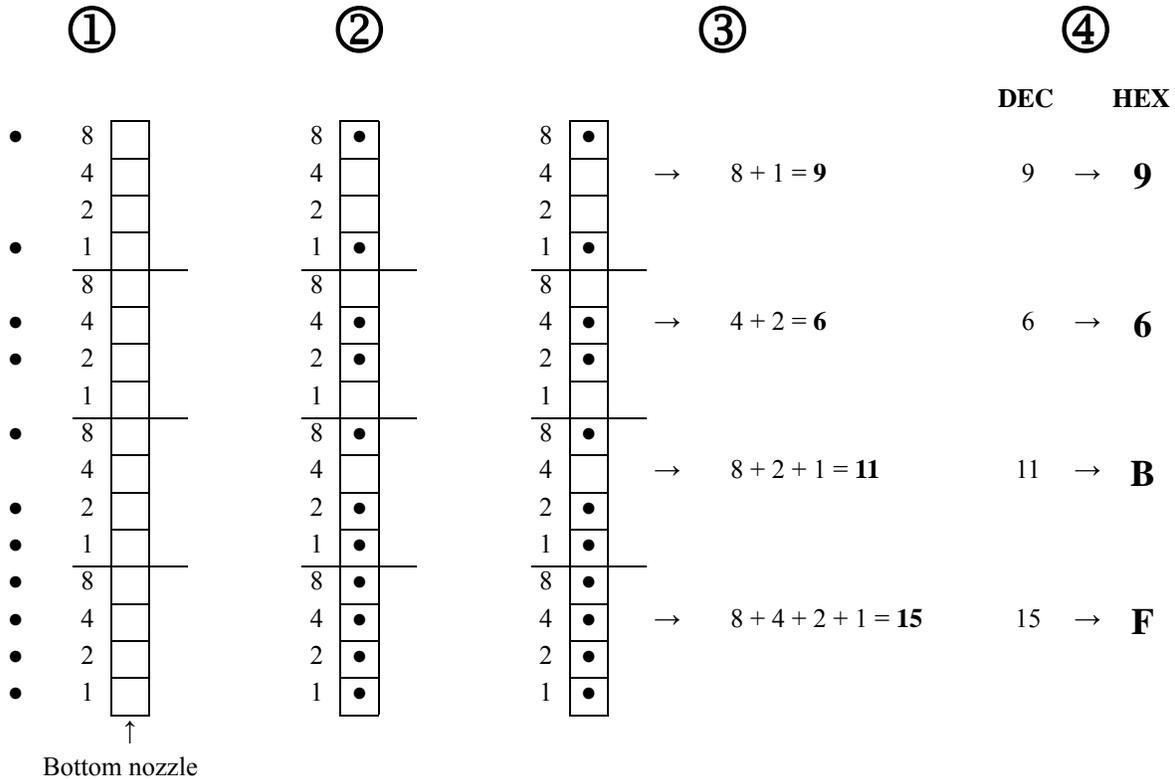
1. Draw and mark a column of squares to represent all the print head nozzles. In this case a 16 nozzle head.
