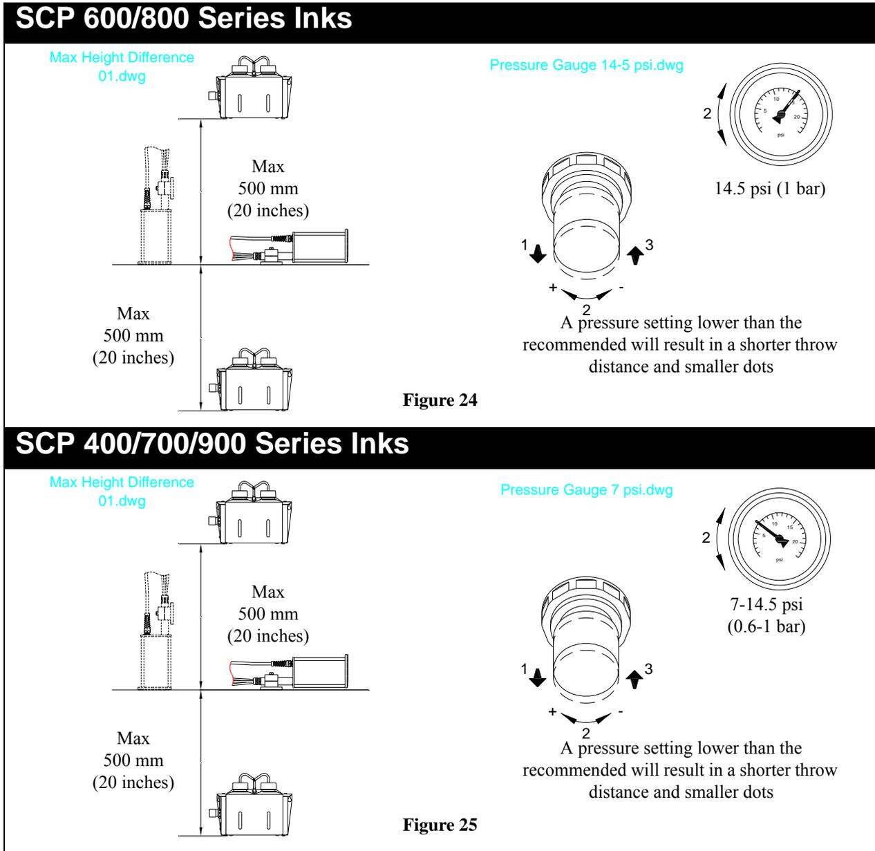
To adjust the pressure of a High Pressure Ink Module, use the following procedure:
