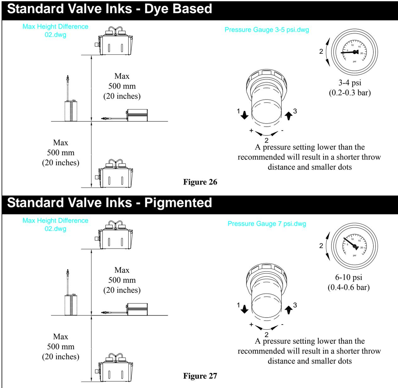
To adjust the pressure of a High Pressure Ink Module, use the following procedure:
