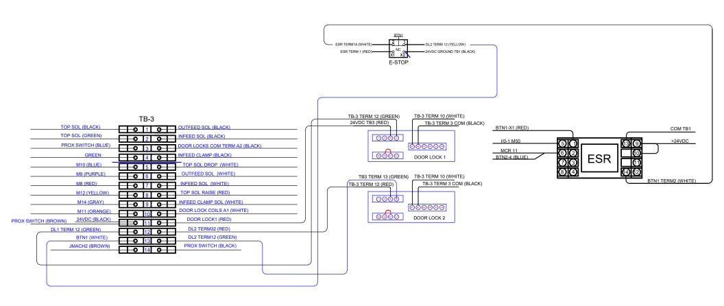
TB-3 TERM 10 IS POWER FROM THE I/O BOARD WHICH UNLOCKS THE DOOR THE CONTACTS ON THE SAFETY SWITCH ARE WIRED WITH POWER COMING IN FROM TB-1 AND EXITING TO THE E-STOP BUTTON TERM!
