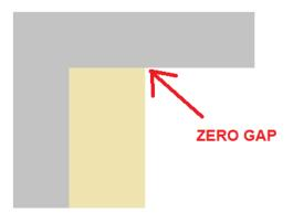
7) Using the same length test file confirm that the saw is only cutting dust off the front of the board, a piece should not fall. Change "front clean up" under the settings screen to adjust this cut. The "front clean up on the main screen is a temporary clean up only. Do not adjust this cut here.
