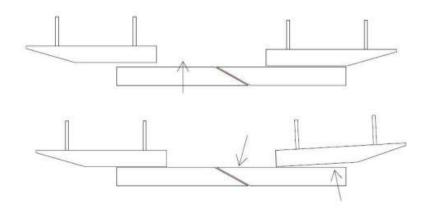
3) Jog a 2x4 into both rollers and check the tension on the table springs. Infeed should have 3/16" gap under the adjustment nut washer, under the outfeed adjustment nuts should be free but very little up and down clearance. Make sure the spring studs are not broken.
