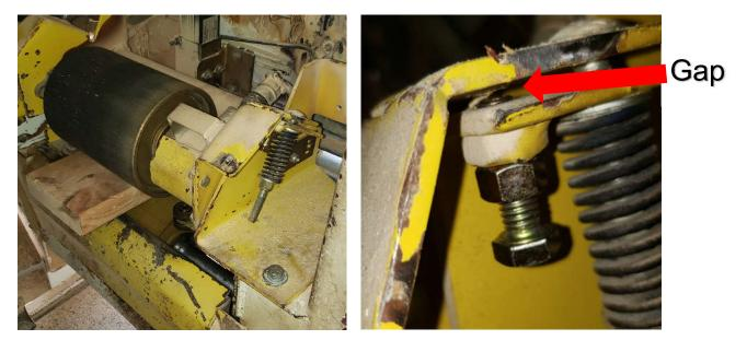
4) You should be able to jog a straight 16' 2x4 thru the saw and the board will stay tight against the fence. When you back the board up, it should ride away from the fence not more than  $\frac{1}{2}$ " in 10 ft of jogging backwards. If it will not do this, the angle of the bottom rollers must be adjusted. It is best to do this one roller at a time. This can be done by using the wedges from the 100 inch test.
