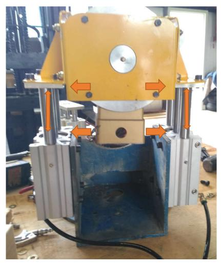
Install cylinders on "starship" mount first. Replace shims that were found during removal.
