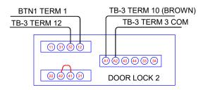
TB-3 TERM 10 IS POWER FROM THE I/O BOARD WHICH UNLOCKS THE DOOR M11=1 THE CONTACTS ON THE SAFETY SWITCH ARE WIRED WITH POWER COMING IN FROM TB-1 AND EXITING TO THE E-STOP BUTTON TERM1
