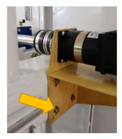
**Step 5)** Test roller by jogging to see if clunk has stopped. If not. Loosen all four bolts on pillow blocks. Roller should rest evenly on both pillow bolts without being bolted down. Tighten bolts in order of below numbers, turning roller to check for smoothness as you tighten bolts. Start with front (closest to door) pillow block 1 & 2. Once the front bearing is tight, confirm there is not gap under the rear pillow block. Tighten 3 & 4 then retest.
