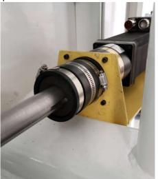
**Step 4)** Loosen 4 bolts on bottom back of motor mount to re center the motor. Retighten Once it has self-centered.
