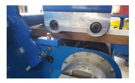
1) Check that taper locks in feed rollers are tight, have 2 bolts each, and that keyways are present with no play
