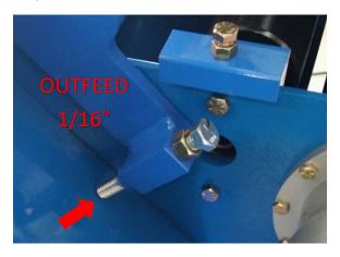
Adjust bolt all the way down, then back off (1/4" = Roughly 3.5 Turns) and (1/16" = Roughly 1 Turn) and lock jam nut in place. Check all four bolts and jam nuts for tightness. Clean the end of each bolt of any compressed sawdust.
