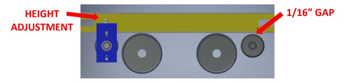
Confirm there is no play in any of the 8 rollers. Also check upper idle roller bearings
