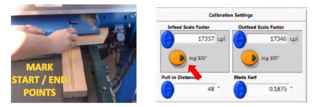
After jogging the board repeat the line with the 2-0-0 board, and measure between the two lines. If your measurement is 100" (8-4-0) it is accurate. If the number is greater or smaller, recalculate your CPI (Counts Per Inch) below:
