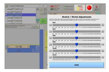
**Note:** Each point represents 1/16". (Example: If 16-0-0 cut is 1/4" short, adjust slider to **-4**) Repeat steps using test board 15-11-0 (90/90) measure result, make adjustment, ect until desired length is achieved.
