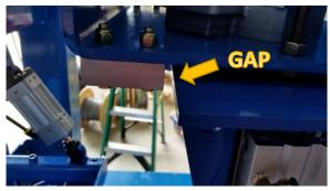
With saw head in the down position (air turned off) and the blade at zero, use a tape measure to check distance between the side of the blade that is facing you and a solid point in the machine. The dust guard at the back door is a good constant surface to use. Then hand rotate the saw head 180 degrees and repeat the measurement on the side of the blade facing you. Both measurements should be equal to each other.
