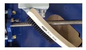
**FEED ROLLERS**: Spray with WD-40 and scrub with a wire brush, thoroughly clean all grooves. Inspect grooves and peaks for sharpness. Light cleaning during shift is suggested.
