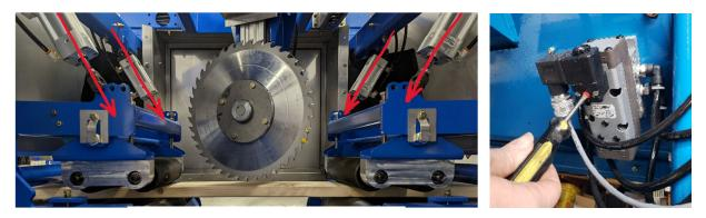
Insert a (straight) 2x4 and clamp in place with both infeed and outfeed.
