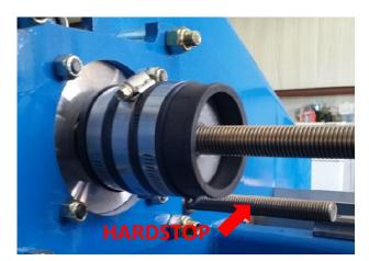
The set screw on ACME side coupling should be lined up with flattened surface on lead screw
