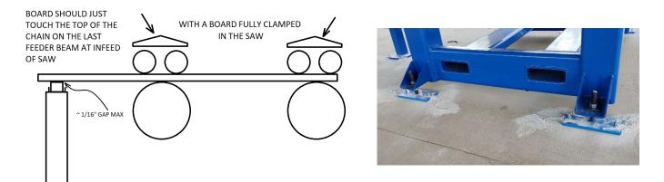
With board still clamped fully in the saw, check first XL-Feeder chain. If board is dragging on chains, the height of the saw needs to be adjusted. Saw should remain level in relation to all four feet. Adjust until board lightly touches first chain with board clamped in both rollers.
