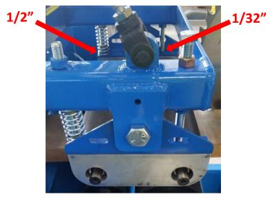
With a board still in saw and the clamps engaged: The spring side gap should be 1/2'' (Two full turns)
