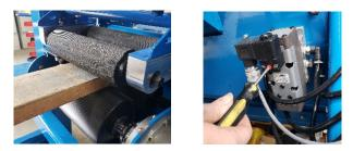
Jog the board forward through the machine, stop before the end of the board. The board should stay tight against the fence.
