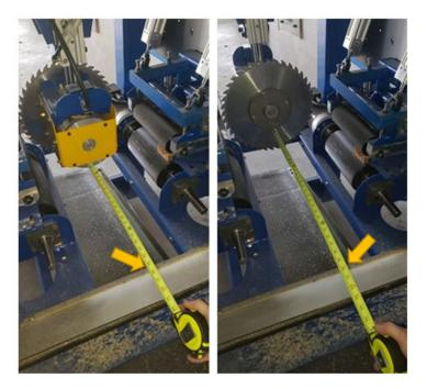
If the measurements are not equal to the previous measurements: Mark the current position of the saw head. Loosen the saw head at its four bolts (two on either side of the carriage cylinder shoe) and move the head half of the distance that the two measurements varied. Tighten bolts and re-measure to confirm the blade is centered.
