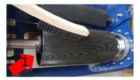
**IDLE ROLLERS:** Spin each of the (6) upper and lower idle rollers. Rollers should spin freely with no lateral play. Replace bearings if any resistance or play is found. Failing bearings can cause expensive shaft damage.
