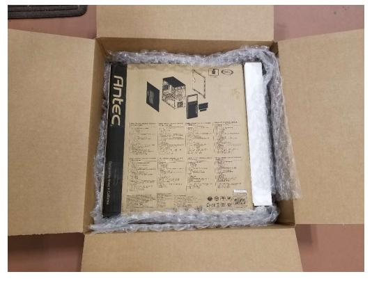
NOTE: FEDEX & UPS ADVISE THAT SHIPMENTS BE PREPARED TO WITHSTAND A MINIMUM 4' FALL DO NOT USE PACKING PEANUTS AROUND CASE, SMALL PIECES OF PACKING CAN GET INSIDE THE CASE
